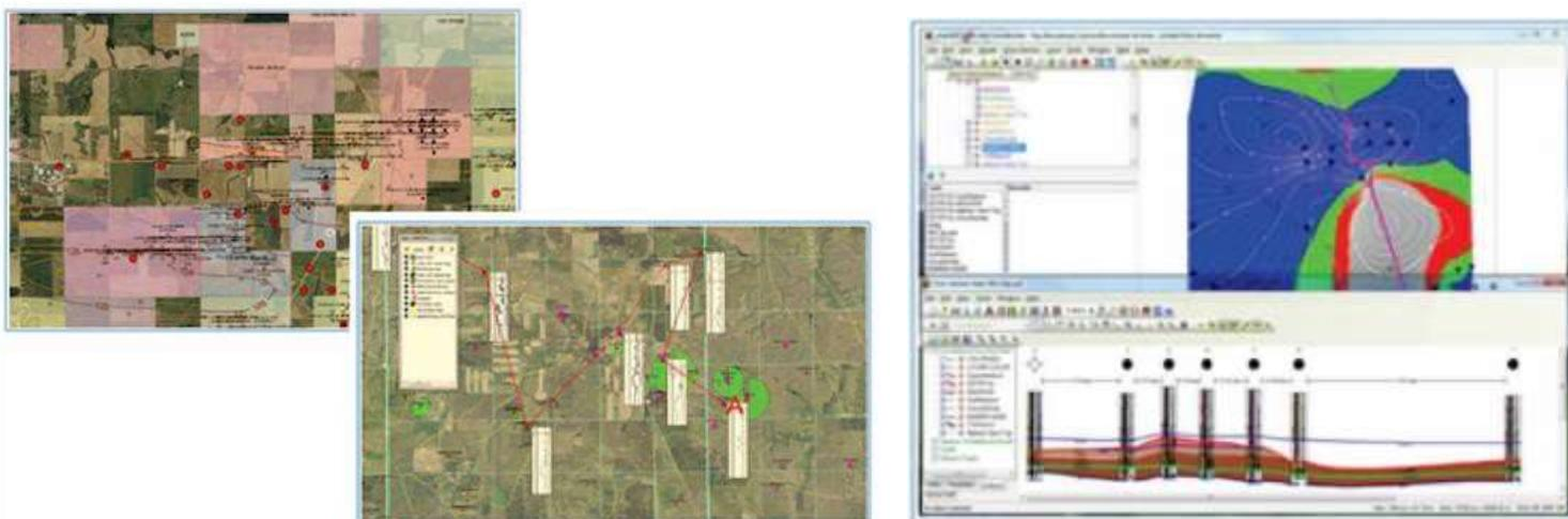
**IsoMap:** Powerful surface gridding and contouring application that combines a wide variety of gridding algorithms and multiple data sources into a single surface or attribute layer.
