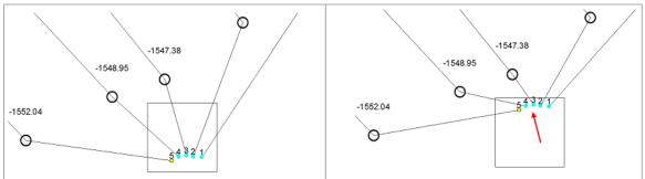
Select multiple well sticks using the <Ctrl> key and right-click. Set the XOffset and YOffset distance to place the selected well sticks at a new location on the map. You can also select and drag and drop multiple well sticks to a new location.
