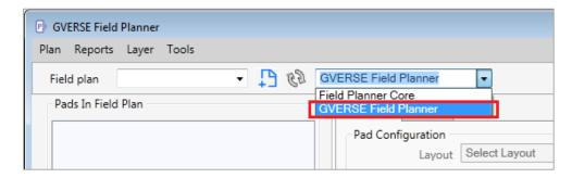
The GVERSE Field Planner features display in the window. You can use **GVERSE Field Planner** to optimize and configure automatic field plans, and manually plan fields using the **Field Planner Core** features.
